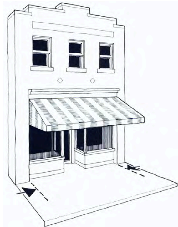
Awnings should always be located below the storefront cornice and between the storefront piers or pilasters.
