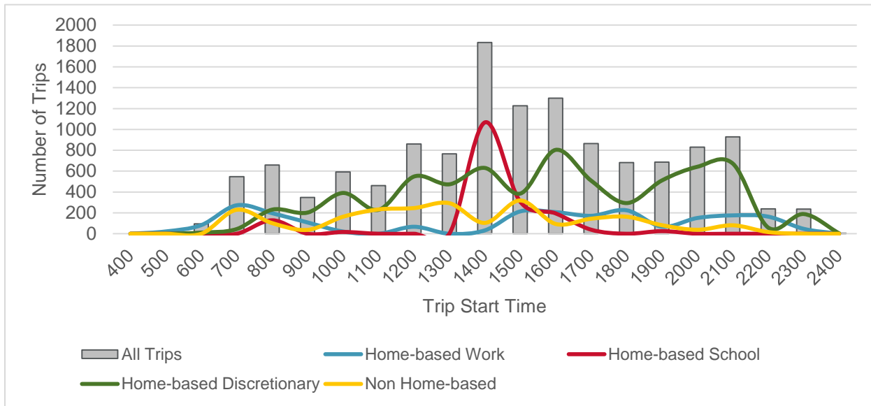
Figure 3-10: Number of Trips by Start Time and Trip Purpose for Secondary Plan Study Area
