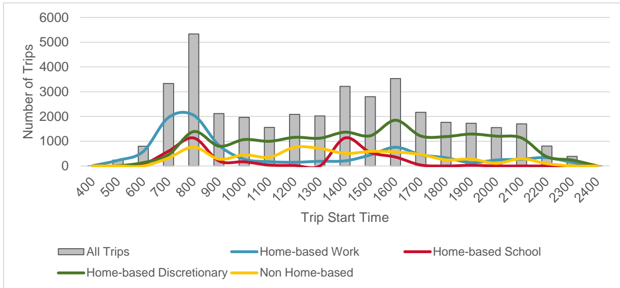
Figure 3-9: Number of Trips by Start Time and Trip Purpose for the Transportation Study Area
