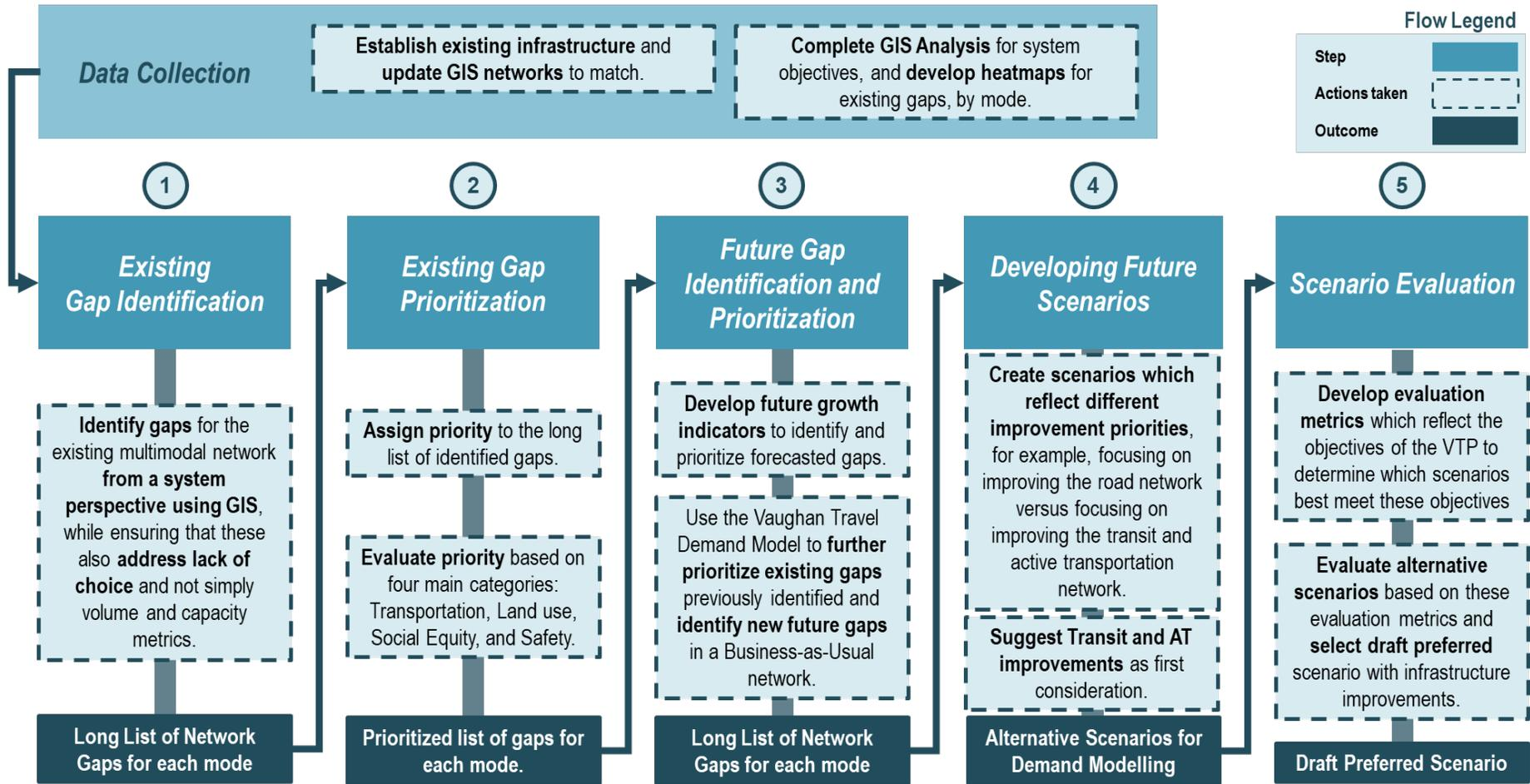
Figure 2-1: Process for identifying gaps and proposing infrastructure improvements
