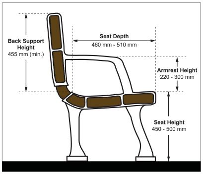
Figure 23: Typical Accessible Bench Dimensions - Section View
