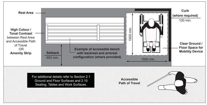
Figure 16: Rest Area - Plan View
