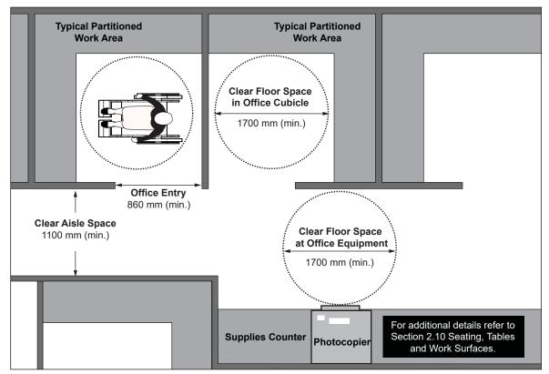
Figure 92: Common-Use Work Areas - Plan View
