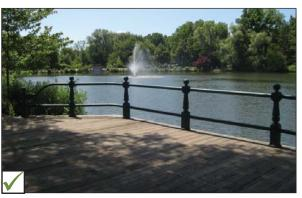
*Example of protective barrier where there is a large elevation change or trail is adjacent to water feature.*
