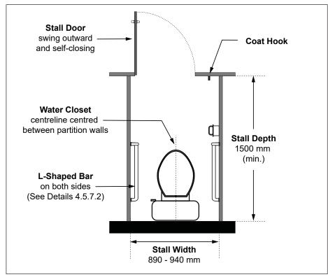
Figure 54: Ambulatory Water Closet Stall or Enclosures
