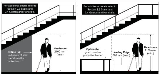
Figure 14: Protection Options Underneath Stairs
