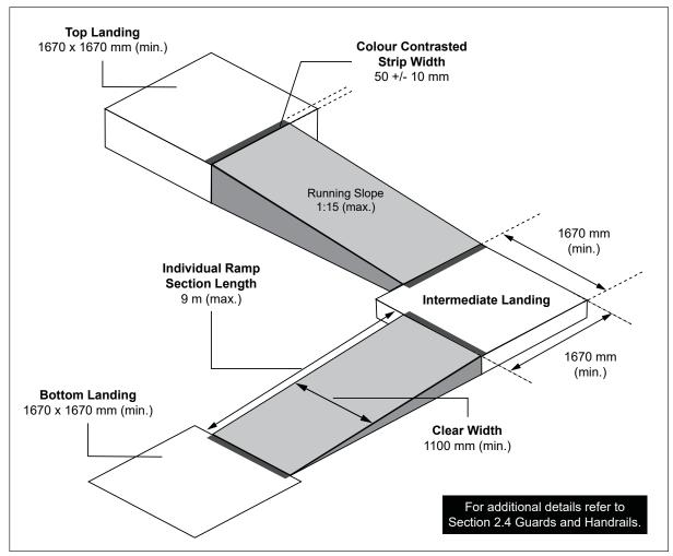
Figure 3: Ramp Design Features
