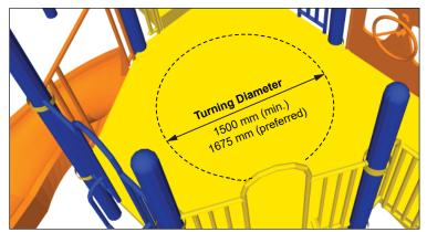
Figure 106: Turning Space - Plan View
