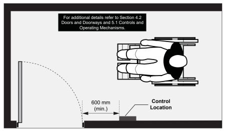
Figure 68: Proximity Card Reader Location - Plan View
