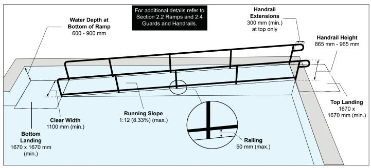
Figure 93: Sloped Entry or Ramp to Swimming Pool
