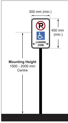
Figure 29: Passenger Loading Zone Vertical Signage
