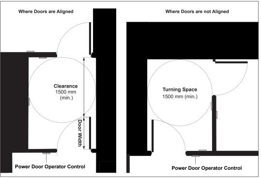
Figure 45: Doors in Series - Plan View
