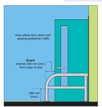
Figure 43b: Guard at Door - Elevation View
