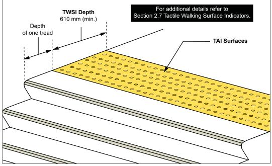
Figure 11: TAI Surfaces at Top of Stairs
