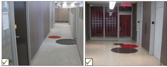
Examples of floor surface and elevator door finishes that minimize glare.
