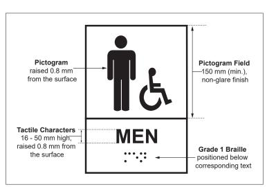
Figure 75: Signage with Tactile Features
