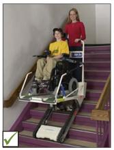
Example of portable elevating device, with platform designed to accommodate mobility aid during evacuation.
