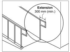
Figure 7a: Handrail Returns to Guard or Rail
