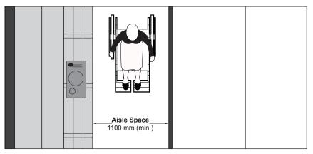
Figure 83b: Aisle Width - Plan View
