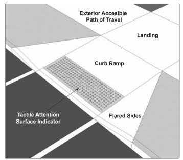
Figure 34a: Curb Ramp with Flared Sides
