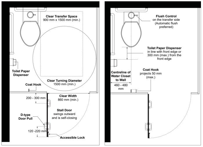
Figure 55a: Water Closet Stall - Space Requirements
