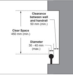
Figure 13b: Handrails in Recessed Area - Section View
