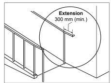
Figure 7b: Handrail Returns to Wall
