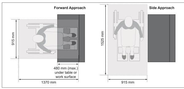
Figure 24b: Clear Floor Space Requirements and Approach at Tables and Work Surfaces - Plan View
