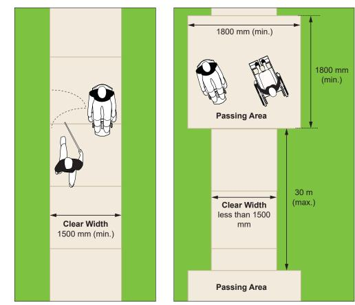
Figure 30a: Minimum Clear Width of Exterior Path of Travel
