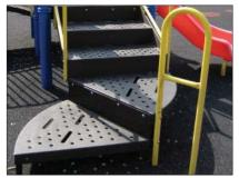
Transfer system to connect elevated play components.
