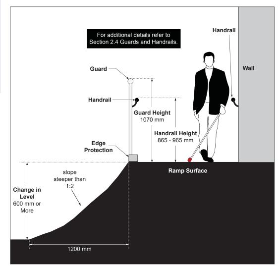
Figure 9: Guard Provision at Ramp - Section View
