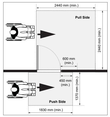
**Figure 44e:** Hinge Side Approach at Side-Hinged Door - Plan View
