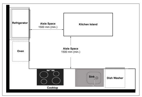
Figure 86: L-Shaped Kitchen - Plan View
