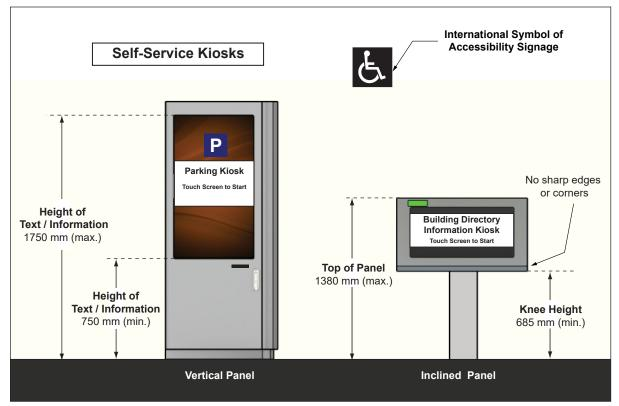
Figure 77: Self-Service Kiosks - Elevation View
