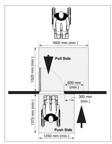
Figure 44c: Front Approach at Side-Hinged Door - Plan View
