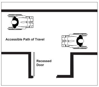
Figure 43a: Recessed Door - Plan View
