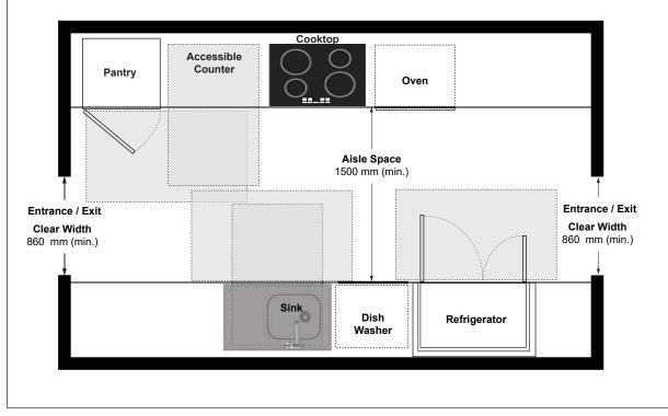
Figure 84: Pass-Through or Galley Kitchen - Plan View
