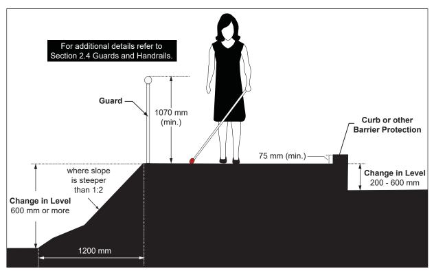
Figure 32: Changes in Level - Edge Protection and Guard Requirements - Section View
