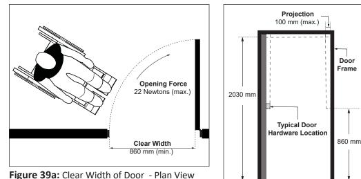
Figure 39b: Clear Width of Door -Section View
