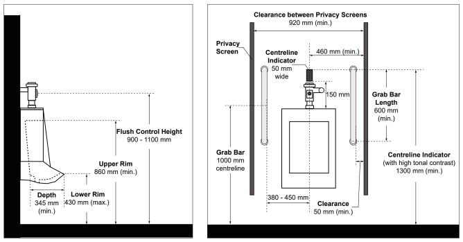
Figure 62a: Urinal - Side Elevation View
