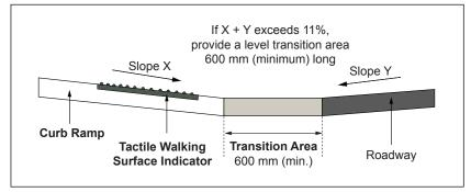
Figure 33: Transition Area - Counter Slope
