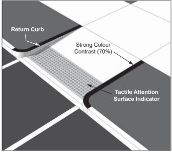
Figure 34b: Curb Ramp with Return Curb
