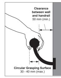
Figure 13a:Handrails on Wall -Section View
