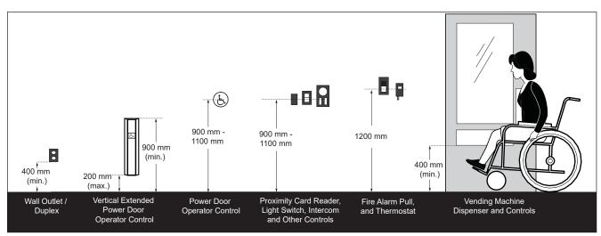
Figure 66: Control Mounting Heights - Elevation View
