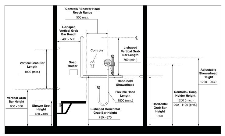
Figure 64: Shower Design and Layout - Section View
