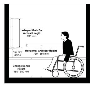
Figure 95b: Accessible Changing Stall -Elevation View
