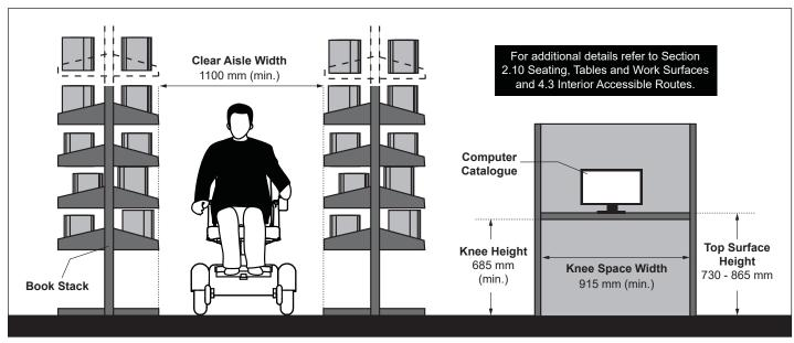
Figure 91: Book Stacks and Accessible Workstation - Elevation View
