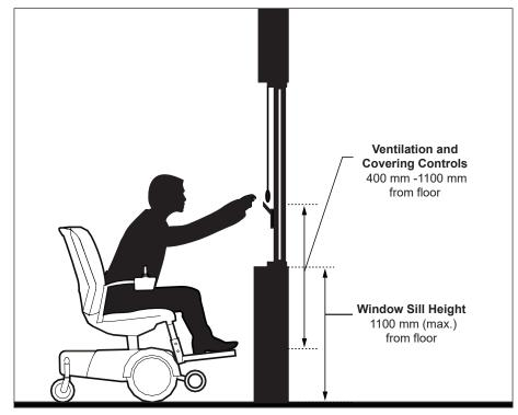
Figure 78: Window Design Features - Elevation View
