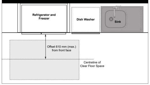
Figure 88: Clear Floor Space at Refrigerators and Freezers
