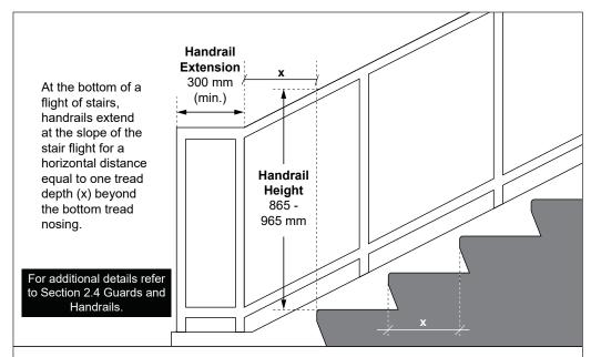
Figure 12: Handrail Extensions at Stairs - Section View
