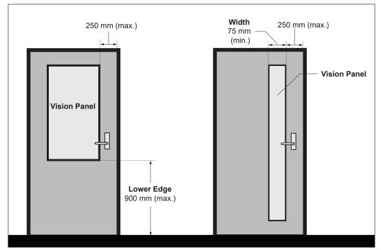
Figure 47: Vision Panels - Elevation View
