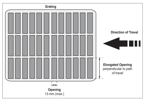
Figure 2a: Grating Opening - Plan View
