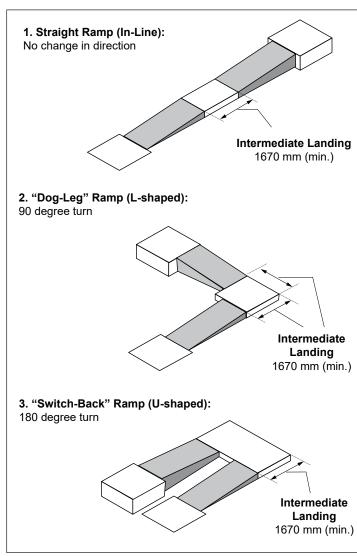
Figure 5: Typical Ramp Configurations
