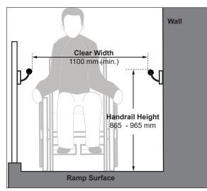
Figure 8: Handrail Design and Features - Section View
