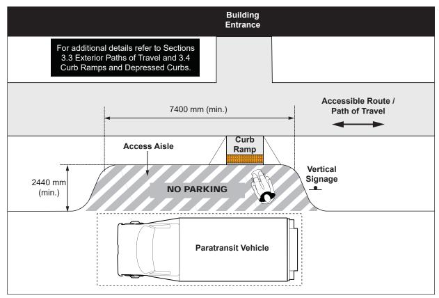
Figure 28: Passenger Loading Zone - Plan View
