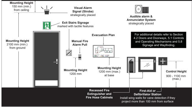
Figure 69: Fire Safety and Evacuation Features - Elevation View
