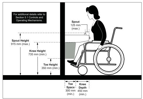
Figure 20: Drinking Fountain Design and Layout - Elevation View
