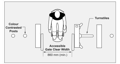
Figure 40: Accessible Controlled Gate
