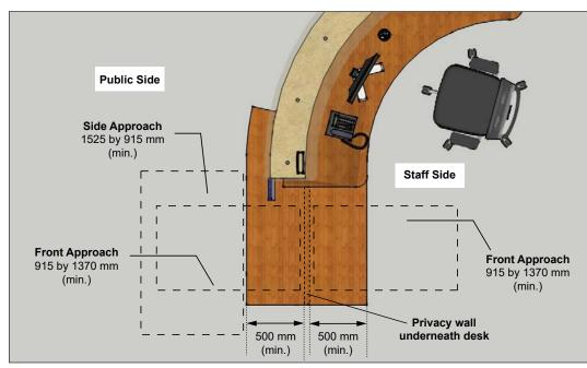
Figure 97a: Clear Floor Space Requirement at Accessible Service Counter - Plan View
