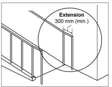
Figure 7c: Handrail Returns to Floor
