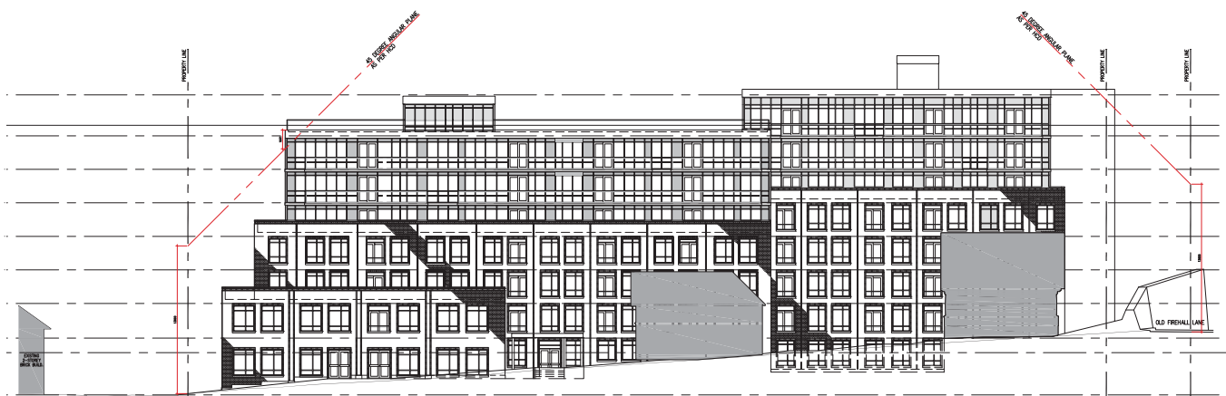
80. North elevation, showing the building generally within the 45-degree setback from 13m as specified by Guideline 6.4.2.2 diagrams by ERA, based on site plan by Architecture Unfolded). For larger scale diagram, see Guideline Study attached as Appendix 7.
