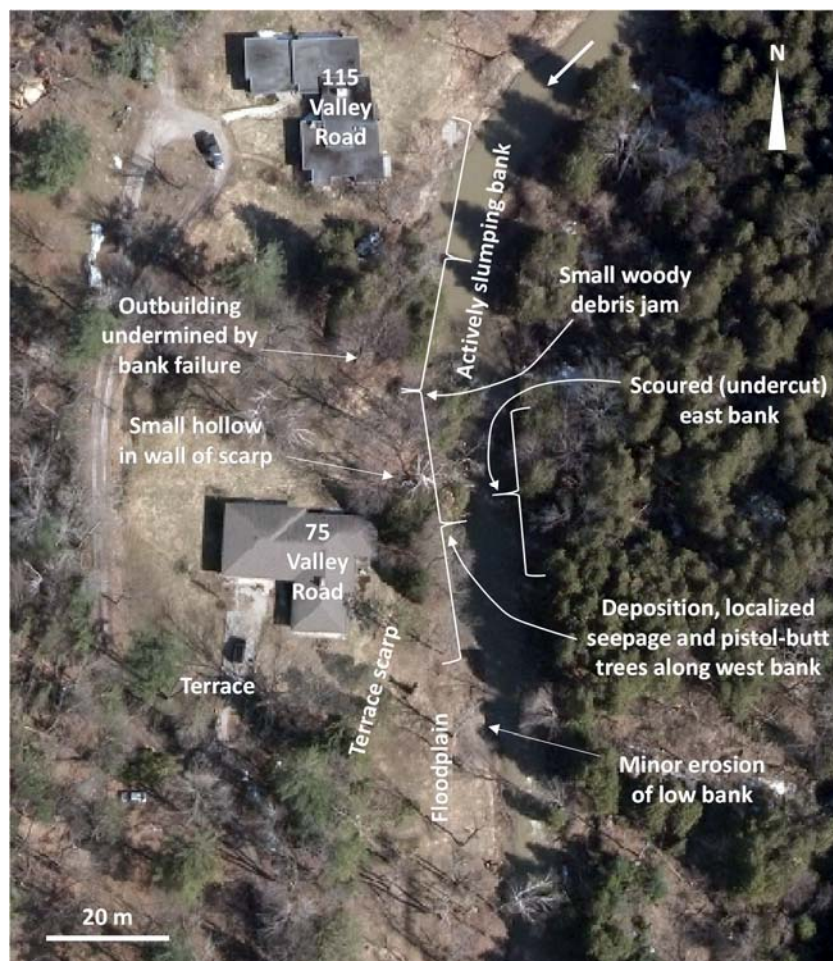
Figure 1. Key features and fluvial processes alongside 75 Valley Road
