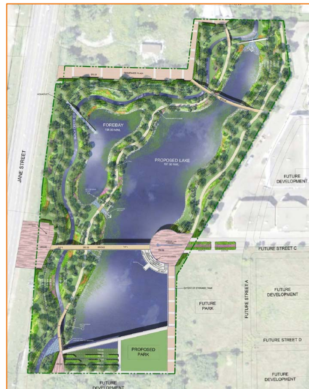
Figure 3 Preliminary SWM Pond Improvements Concept (TMIG/Schollen & Company)
