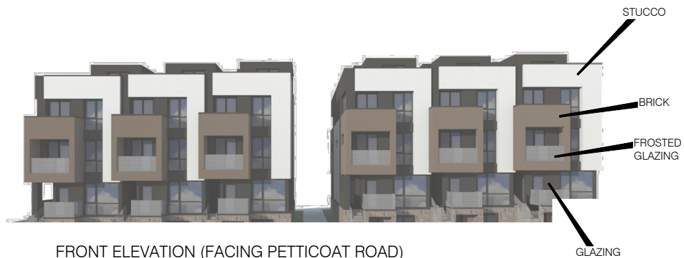
FRONT ELEVATION (FACING PETTICOAT ROAD) (INCLUDES 2 UNITS PER STACK; FIRST FLOOR UNIT AND A UNIT COMPRISED OF 2ND & 3RD FLOORS)
