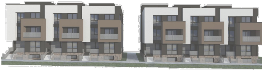
REAR ELEVATION (NORTH) (INCLUDES 3 UNITS PER STACK; BASEMENT UNIT; FIRST FLOOR UNIT AND A UNIT COMPRISED OF 2ND & 3RD FLOORS)
