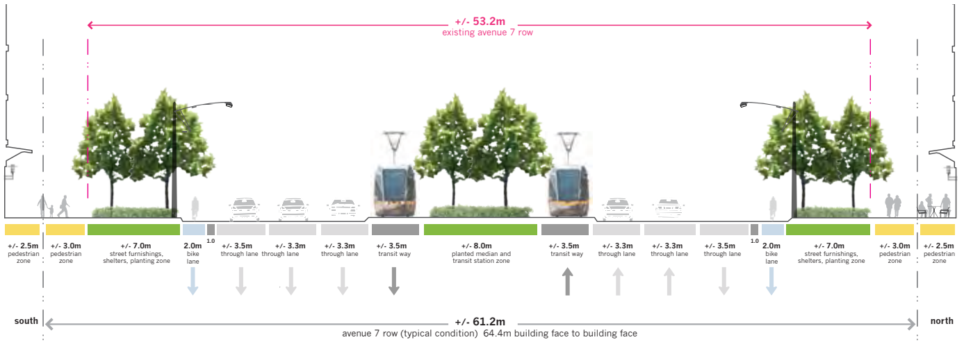
FIGURE A &gt; SECTION OF AVENUE 7 LOOKING WEST (TYPICAL CONDITION)
