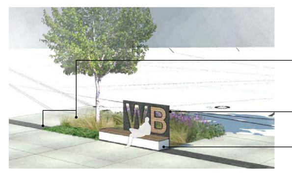
Granite coloured banding - paving type III - and atgrade planting bed incorporated into the gateway plaza
