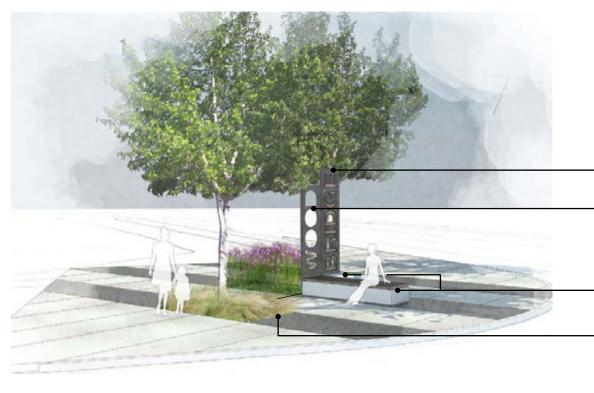
embedded into metal plate [height of 3190mm above bench] Letters cut out from metal plate [height of 2690mm above bench] 2 Custom benches
