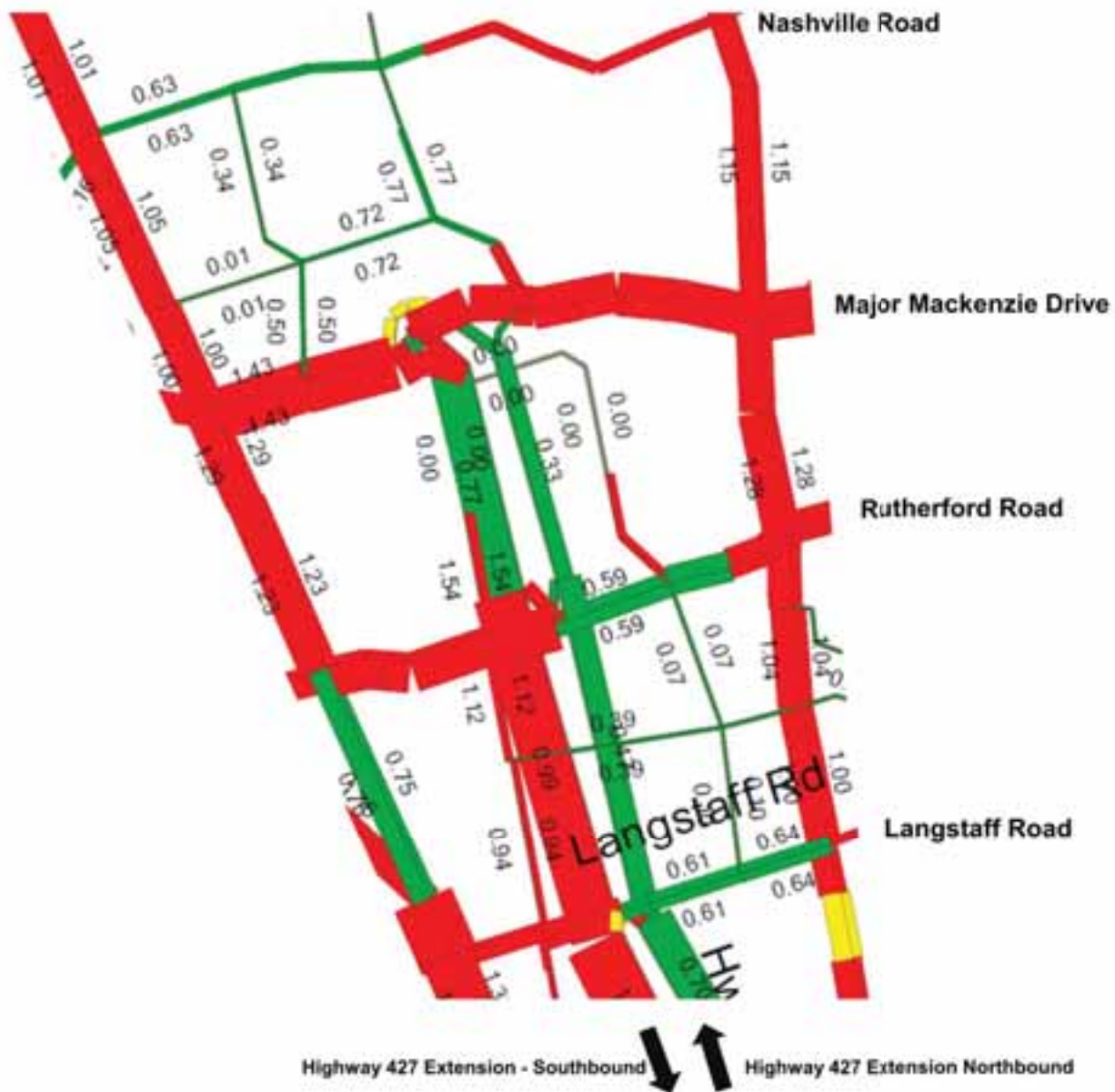
Figure 4. 2031 AM Peak Hour Traffic Congestion Analysis (Volume to Capacity Ratios for Individual Road Segments)
