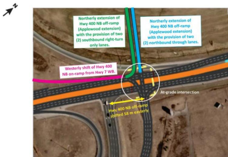
Cost estimates associated with the Highway 400 NB off-ramp, the Highway NB 400 on-ramp, the ramp intersection and drainage requirements were derived. According to the study, the estimated construction cost, inclusive of Minor Items, Contingency, Engineering and HST is approximately \$6,200,000.
