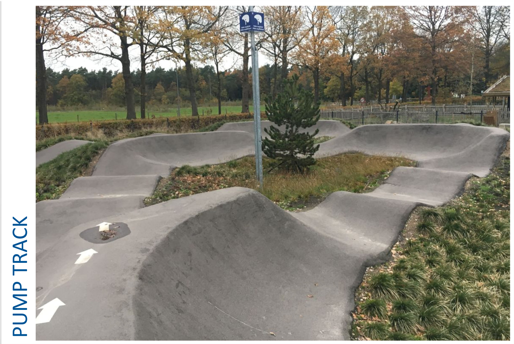
A looping circuit of smooth, raised rollers and berms made of asphalt that allow users to move through the course using a “pumping” motion of their arms and legs.
