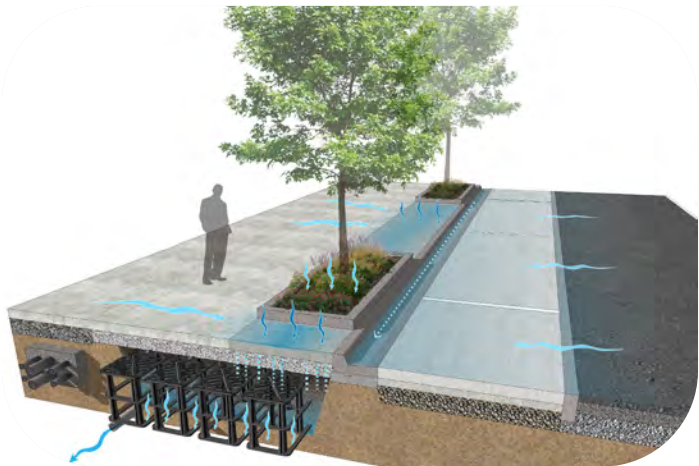
Figure 85. Soil cell technology can promote healthy tree growth.
