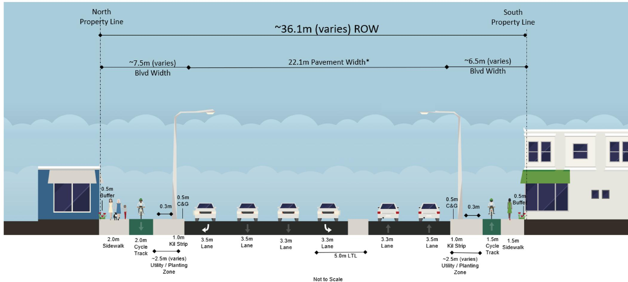
Note: \*Pavement width measured to Edge of Pavement
