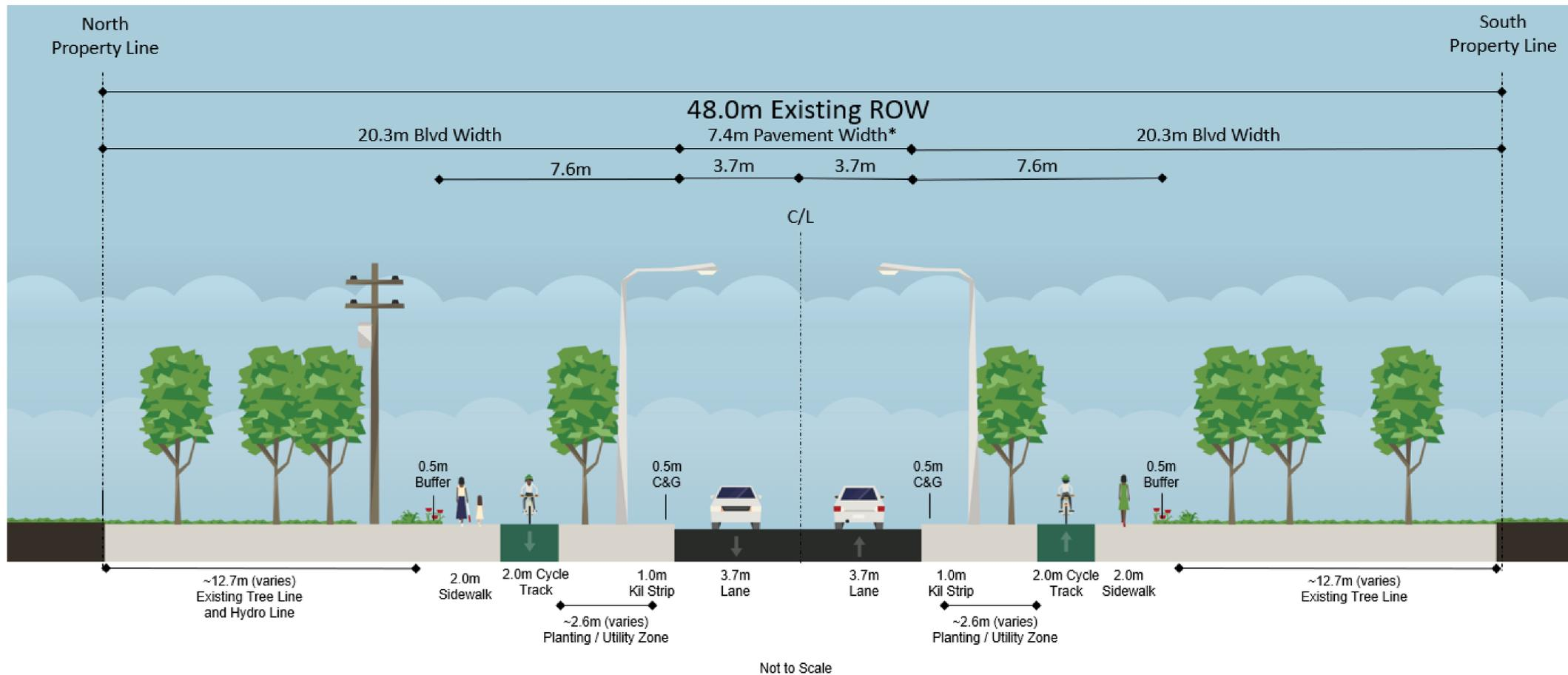
**Note:** 0.6 m buffer between sidewalk and cycle track to be applied where space is available within the ROW
