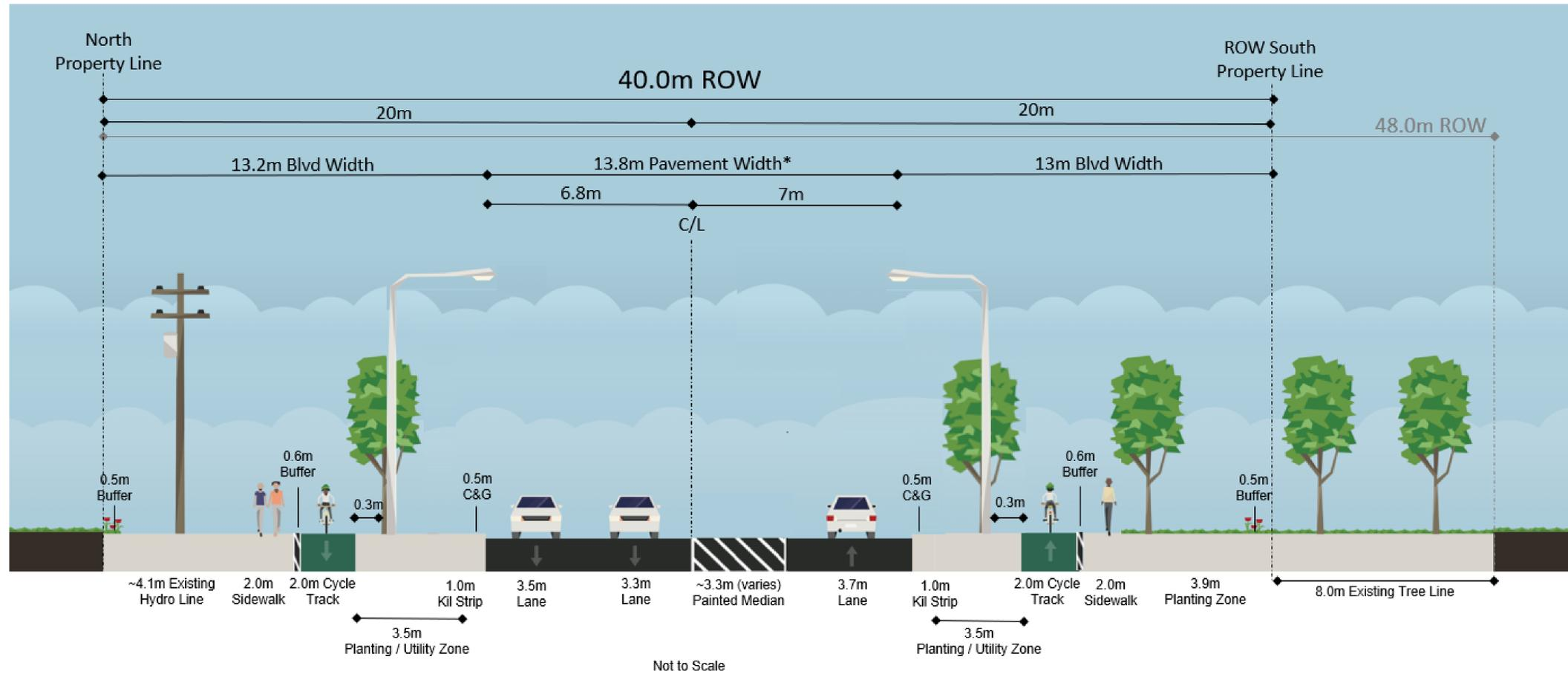
Note: \*Pavement width measured to Edge of Pavement
