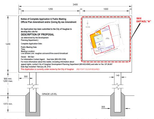
10.4 Below is a dimensioned schematic of a Notice Sign(s) for a CIHA order request
