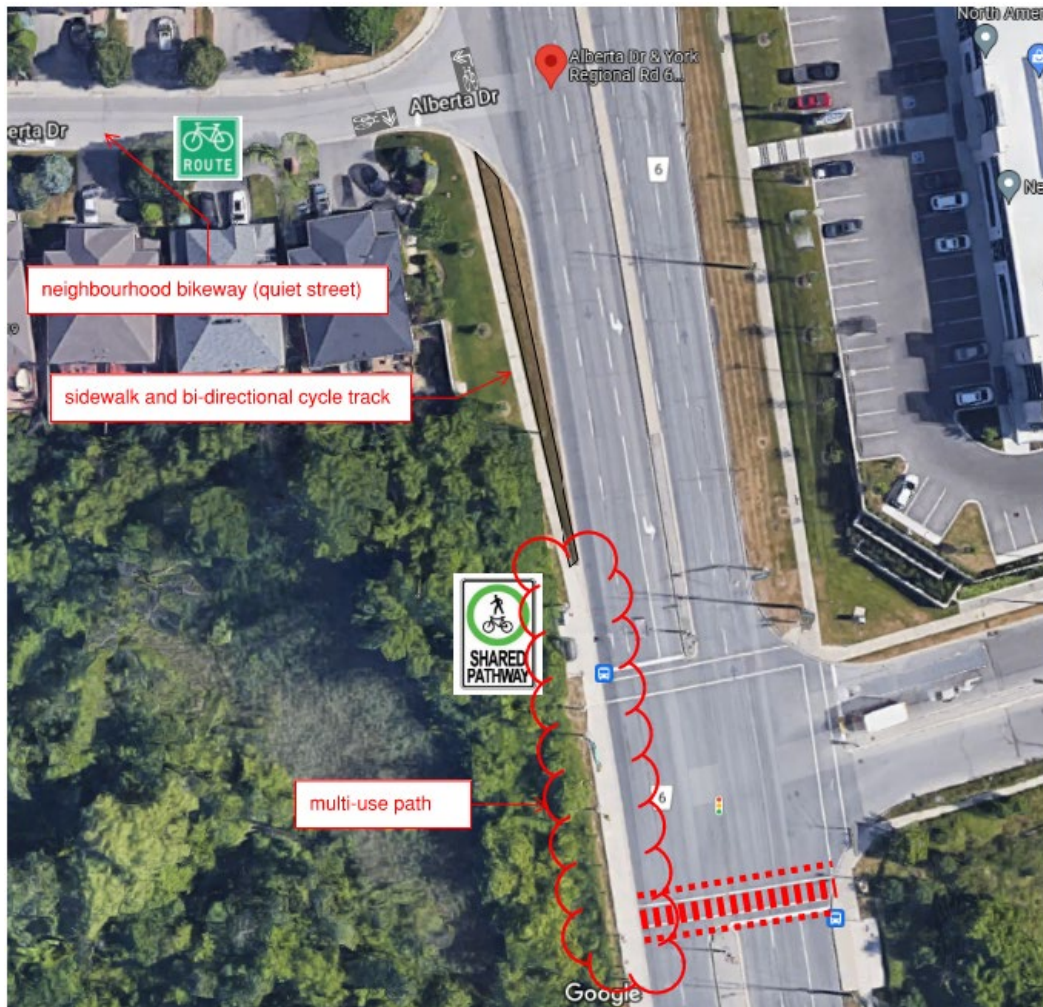
FIGURE 14: CONNECTION ALONG ALBERTA DR. AND KEELE ST.
