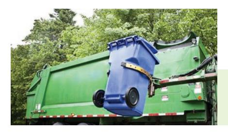
**Automated collection** relies on trucks fitted with mechanical arms to pick up/empty carts into a collection vehicle.
