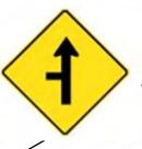
Provision of "Intersection Sign – Controlled" in the northbound direction approaching Pierre Burton. Located a minimum advance distance of 160 metres
