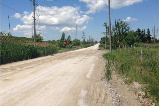
Photo 18: No proper ditching along the gravelly road
