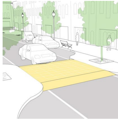
Speed table / Raised Crossing
