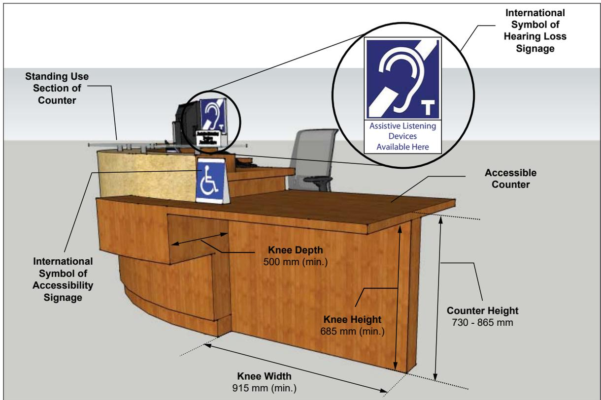
**Figure 97b:** Accessible Service Counter with Knee Clearances
