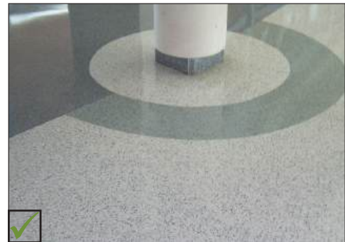
Where structural column / support is within accessible route, colour contrasted floor surface at base is beneficial for all users.
