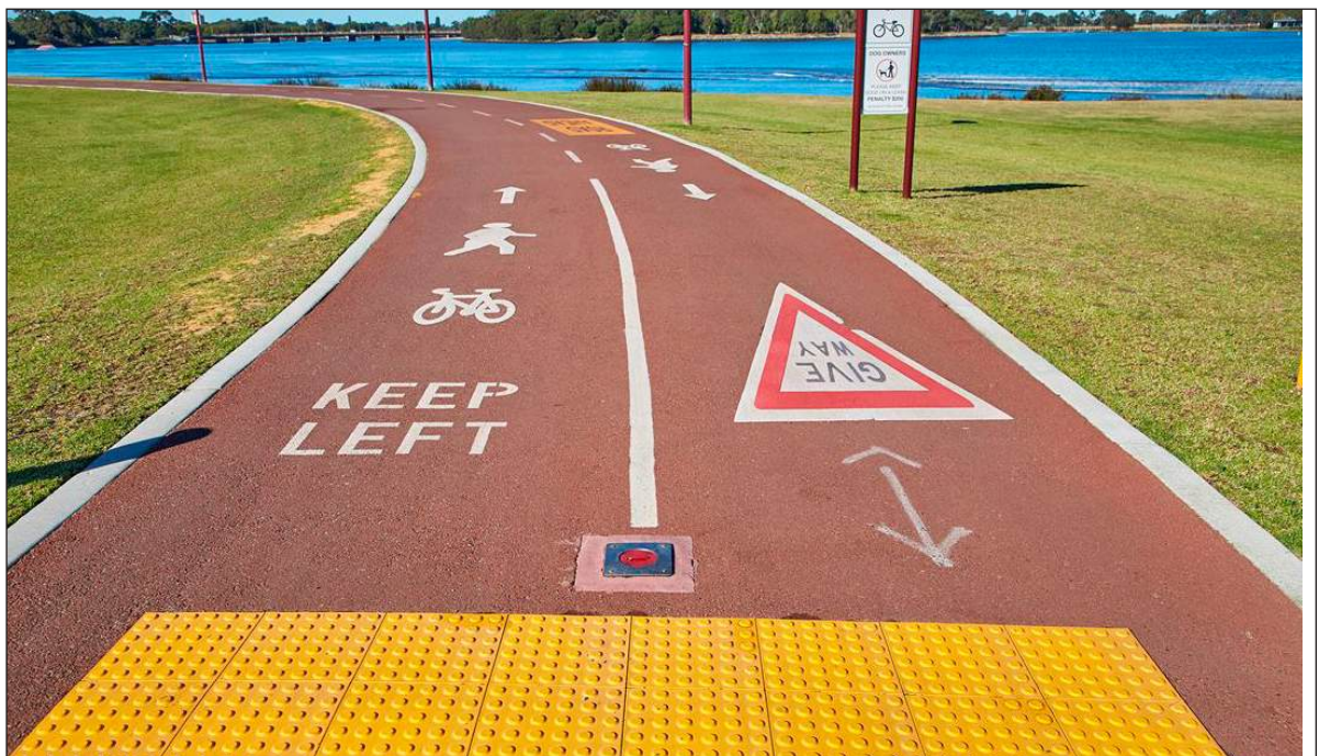
Bike path with tactile warning strip
