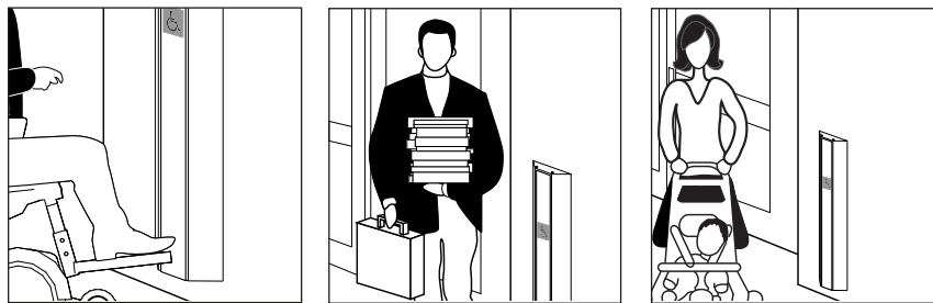
Figure 4: Example of Power Operator Control Promoting Universal Use
