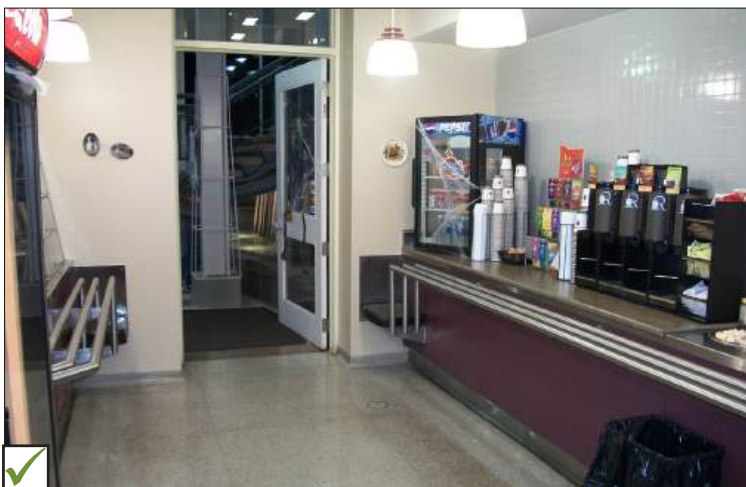
Clear aisle space and knee clearances provided at food displays and tray slides.
