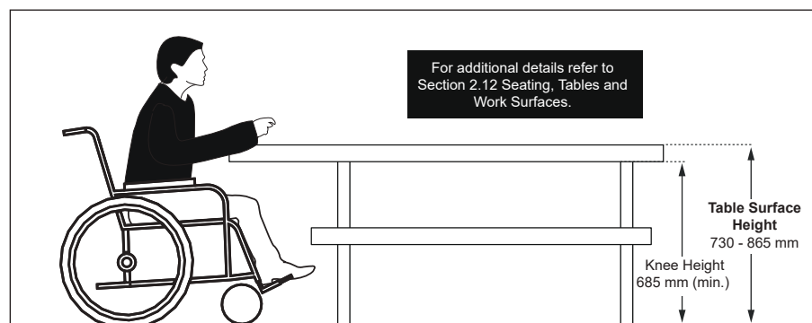
Figure 102b: Picnic Table Design and Features - Elevation View
