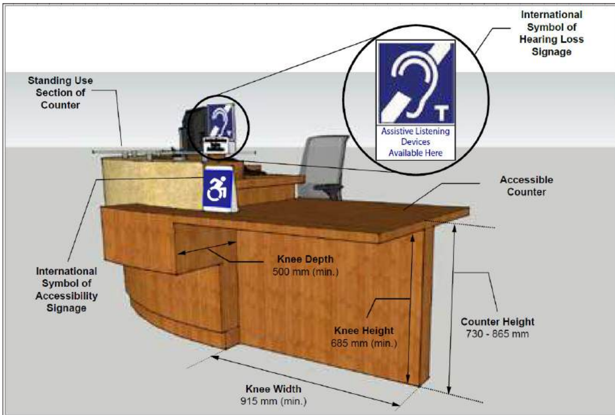
Figure 98b: Accessible Service Counter with Knee Clearances
