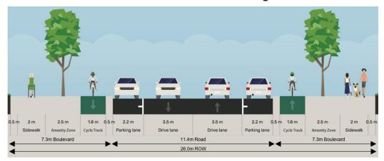
Figure 8-4: Minor Collector Cross Section with Parking on Both Sides – Midblock Pedestrian Crossover
