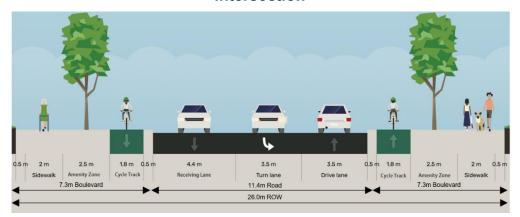
Figure ES - 13: Minor Collector Cross Section with Parking on One Side - Midblock
