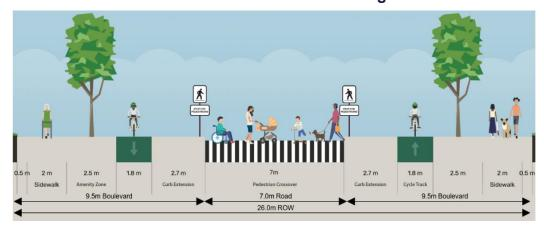
Figure ES - 12: Minor Collector Cross Section with Parking on Both Sides - Intersection
