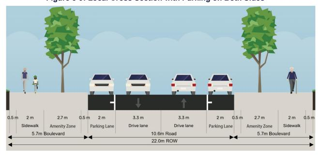
Figure 8-9: Local Cross Section with Parking on Both Sides
