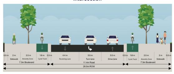
Figure 8-6: Minor Collector Cross Section with Parking on One Side – Midblock
