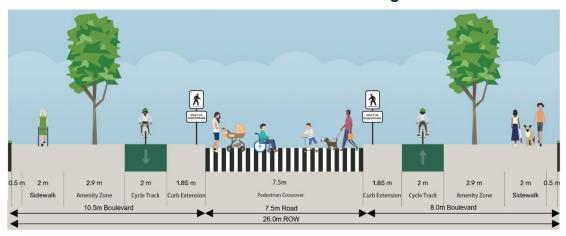
Figure ES - 15: Minor Collector Cross Section with Parking on One Side - Intersection
