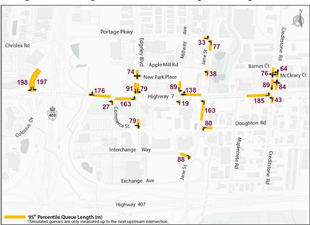
Figure 3-29. Existing 95th Percentile Queue Lengths - Morning Peak Hour
