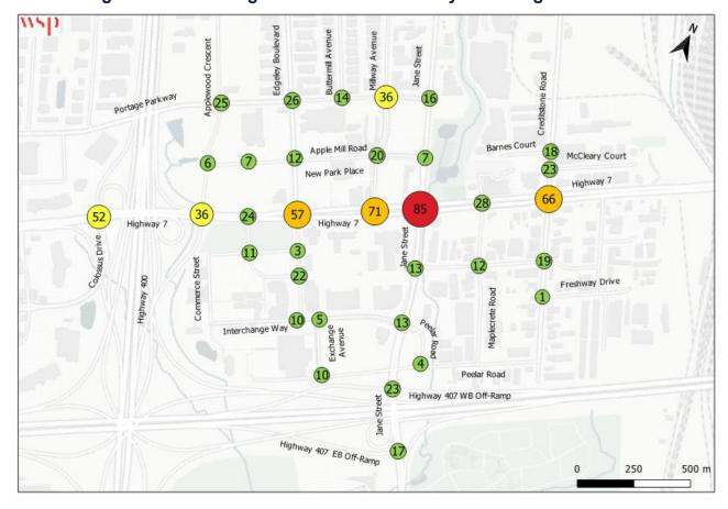
Figure 3-28. Existing VMC Intersection Delay - Morning Peak Hour
