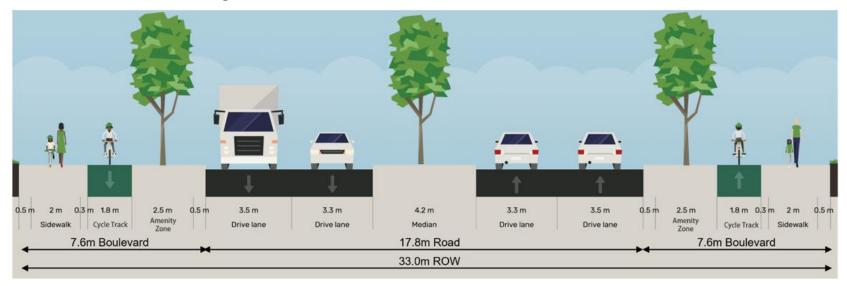
Figure 8-1: Minor Arterial Cross Section - Midblock
