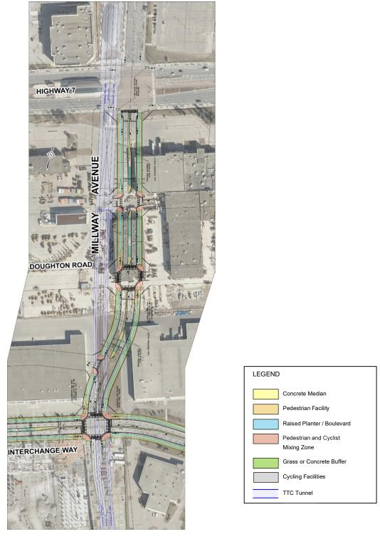
Figure 8-1: Millway Avenue Preferred Alternative Alignment (Option 1)
